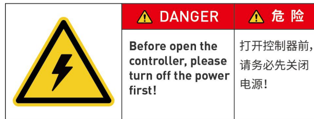
Figure 1- 2 Label to caution preventing electric shock
